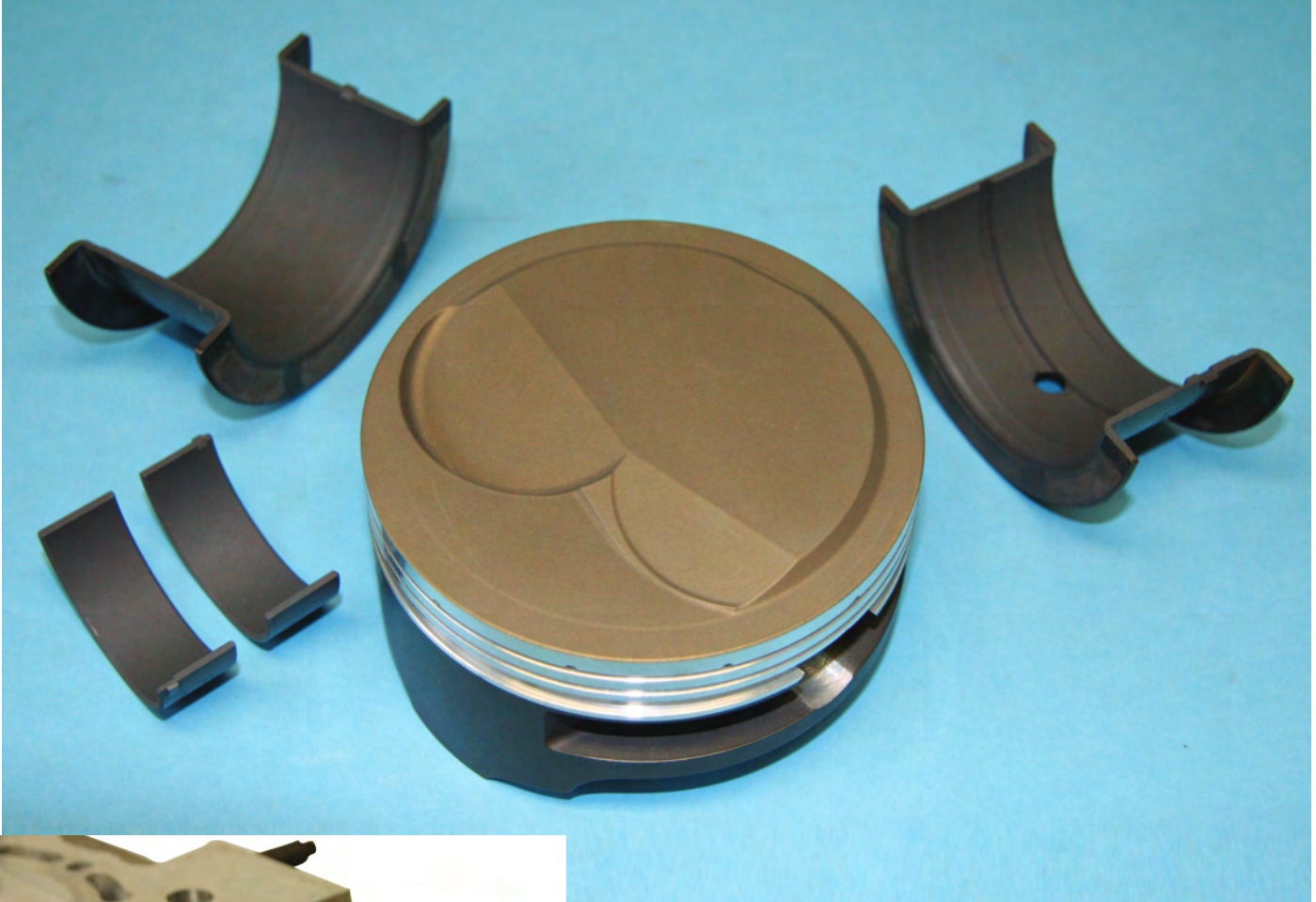
Coatings on pistons, combustion chambers and valves are the internal engine parts that will provide the greatest power gains.
