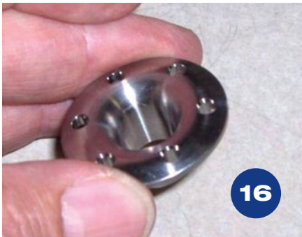
Fig.16: A lightweight steel retainer
