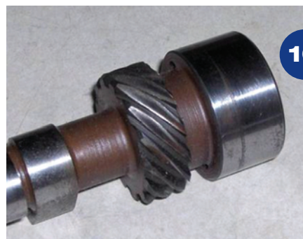
Fig.10: Cam drive gear wear
