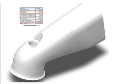
Port volume can be 3D printed instead of making rubber molds but the virtual volume can be solved for average pressure, velocity and other parameters of interest with no slicing, dicing or tracing on graph paper.
