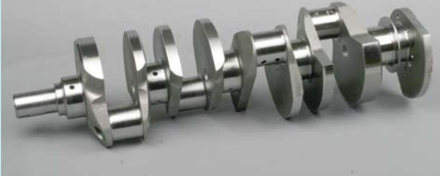
Checking each main journal diameter and record.
