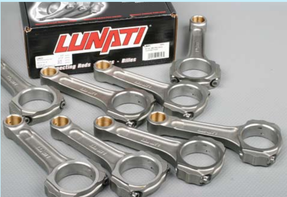
Once all pistons, rods, rings and bearings have been test fitted and assigned cylinder locations, keep them organized.
