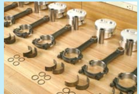
Once all pistons, rods, rings and bearings have been test fitted and assigned cylinder locations, keep them organized.
