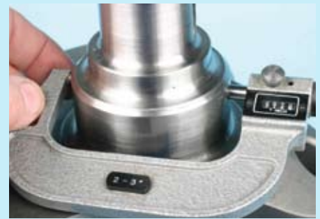
Checking each main journal diameter and record.
