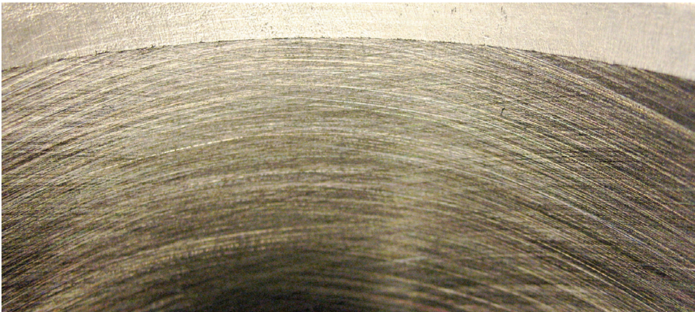
This is a shot of a used Nikasil coated cylinder in the un-run portion. If you look at the portions to the far right and left you can clearly see the very uniform crosshatch pattern.
