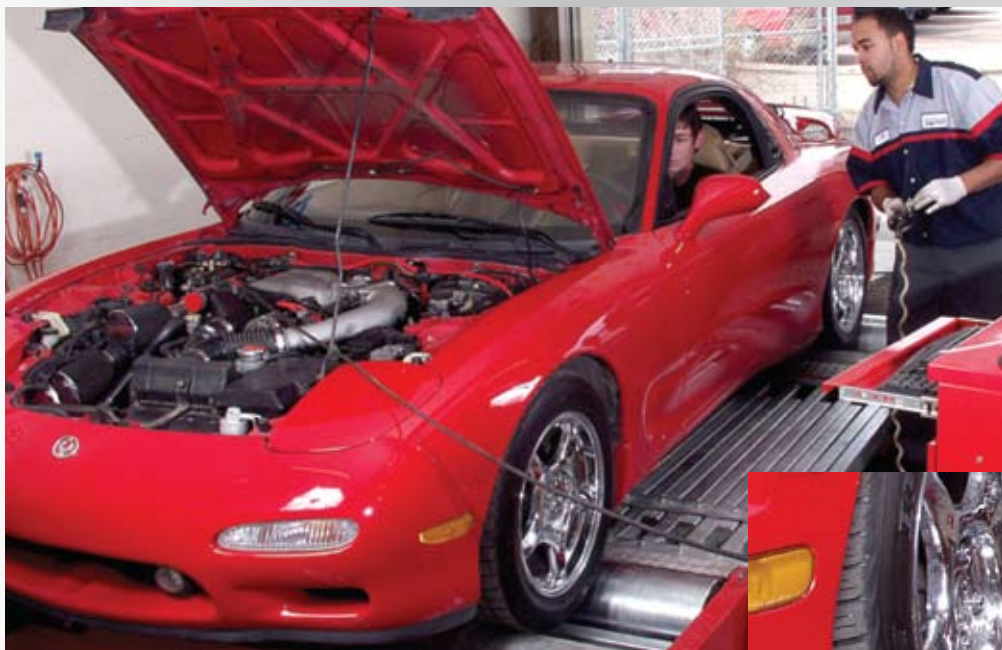
LEFT: Hot rod Mazda with twin turbos is on the chassis dyno to verify tune-up work without the liability of test driving on the streets. Technician on the right has command of the dyno and communicates with the driver during the test.
