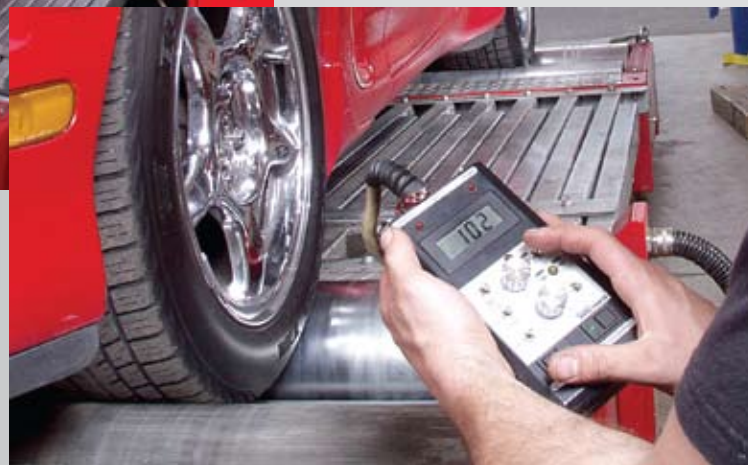
BELOW: The handheld controller on this AWD chassis dyno allows the operator to command all sorts of things including changing the wheelbase. The dyno can be commanded inside or outside the vehicle being tested.
