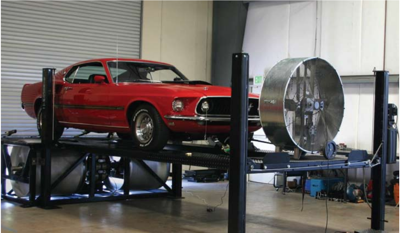
This muscle Mustang is on a large roll dyno about to be tested. The Mustang is on a lift so the dyno can be mounted above floor line. The dyno uses an eddy current power absorber in between the drive rolls. Large rolls are better for either high power or for endurance testing. The fan shown is for short tests only. Longer tests require lots of airflow.
