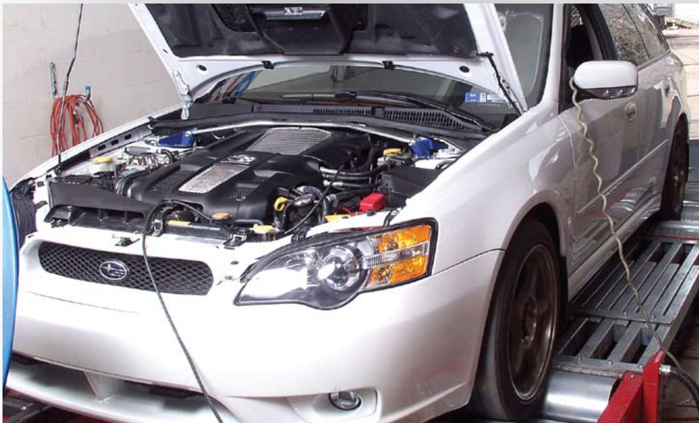
Typical testing for improving the tune up on grocery getters is a normal application for chassis dynos. This photo shows an AWD Subaru wagon undergoing a power test.
